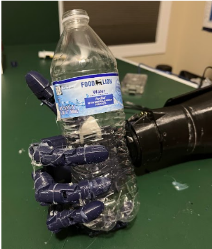
Figure 10: Above is the arm tested for a common object such as a water bottle.
