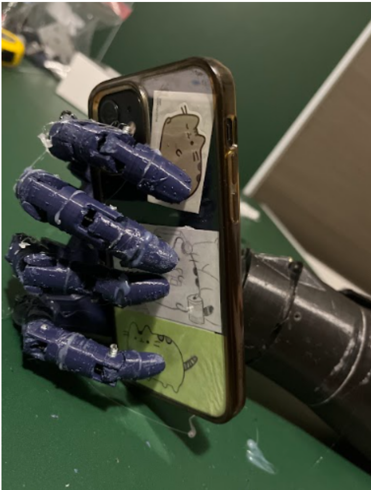
Figure 8: Above is the arm being tested for a common object such as the phone.
