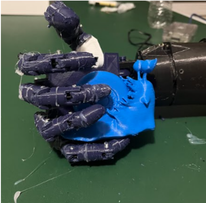
Figure 9: Above is the arm being tested for a common object such as a Minifigure.
